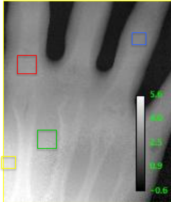
Proton Radiograph (directly in RSP) with 0.5x0.5 mm pixels
