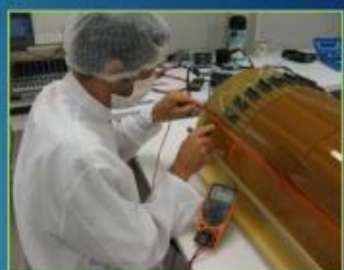
Electric leak test
