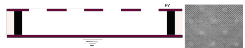
Figure 2. Left: Kapton pillars are created with a step of about 500 microns; Right: photo of a mesh with copper spots used to protect the polyimide below during etching in order to form the pillars.
