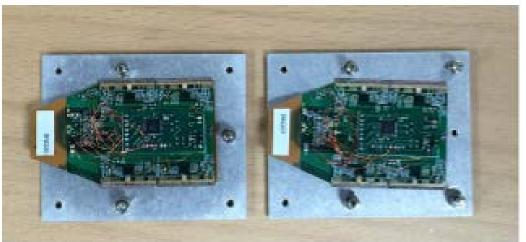
Prototype Quad Modules (basic building block of phase-2 Pixel layout) using FE-I4 chips and prototype CIS n-in-p sensors.
