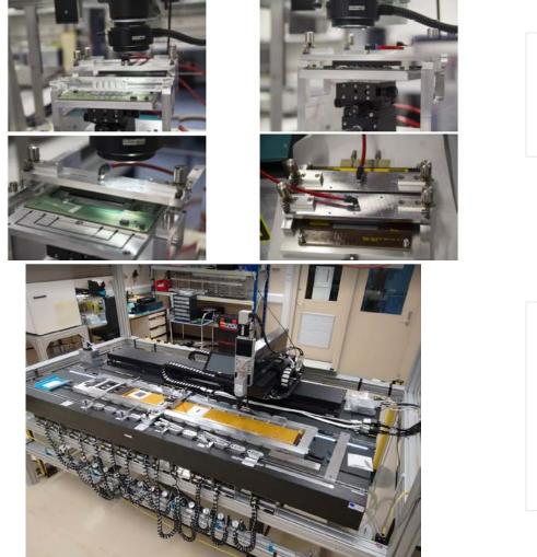
Module assembly tooling developed on dummy modules, being used now for prototype modules.
