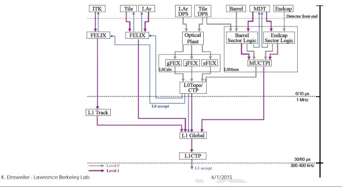
Note: L1 Global needs to provide capability for processing roughly 40 events in parallel.
