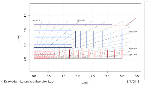
Initial simulation studies based on idealized layout in very forward region using pixel disks extending to  $\eta$ =4.0
