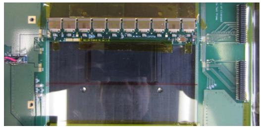
Complete module with 10 ABC130 chips on hybrid (2560 ch), with HCC controller chip, and shortstrip (24mm) sensor.
