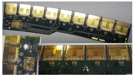
Complete endcap hybrid with ABC130 FE chips and HCC controller chip.
