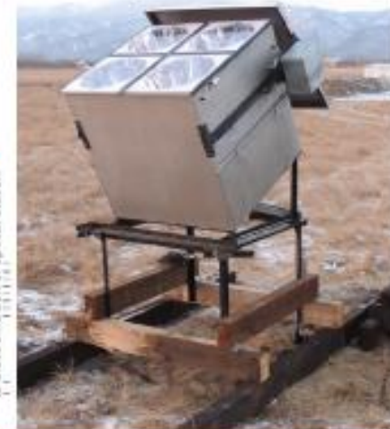
Optical detector of Tunka-133
