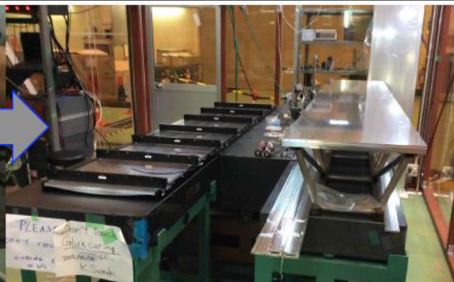
QBB: strong back flattening, button & enclosure gluing.
