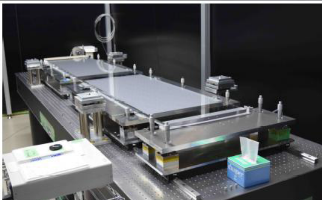
Optics: alignment, gluing, curing and aging (~2 weeks).
