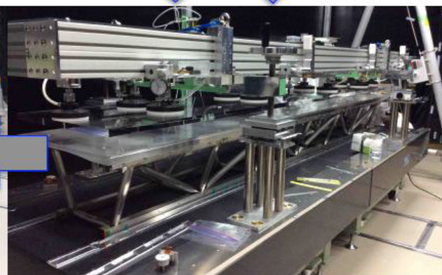
Move optics to QBB using the "lifting jig".
