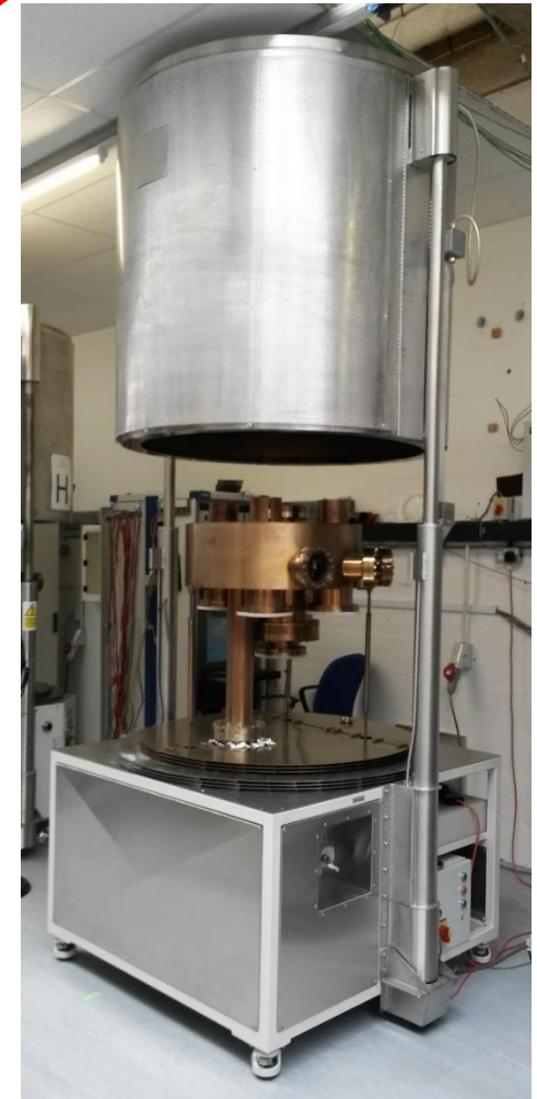
New process rig and oven to produce 3 square tubes
