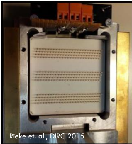
Photonis, 45x45mm, 3x100 Anodes, 0.5mm pitch
