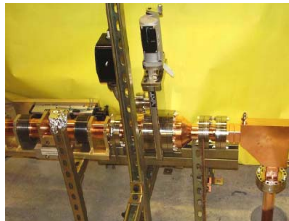
The uncompressed arm has a variable phase shifter and a gate valve
