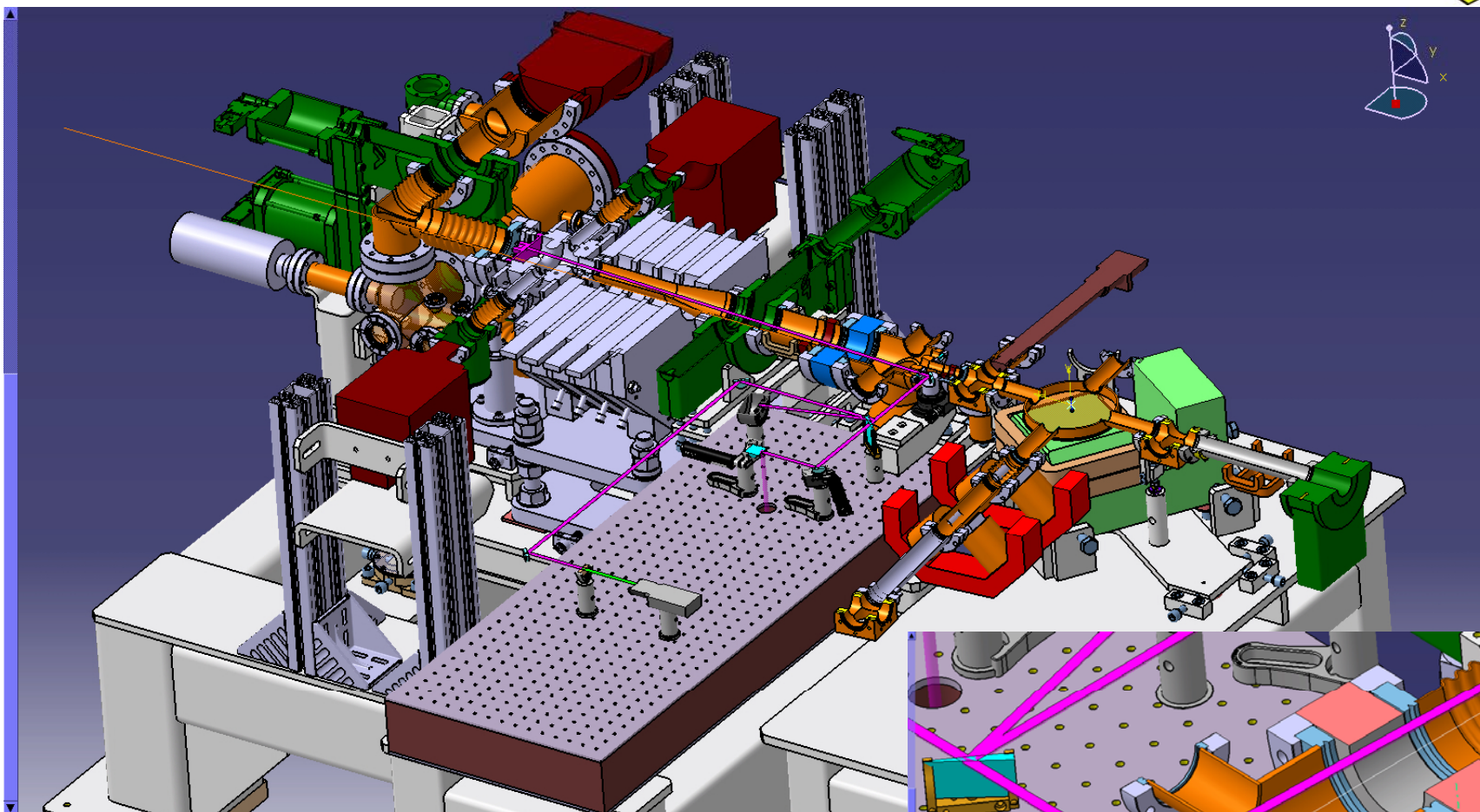
Cut view of the Photo-injector
