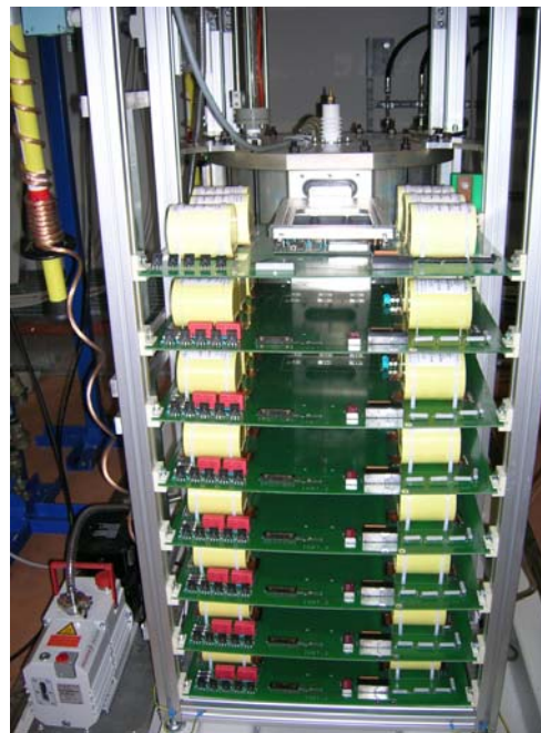
IGBT PCBs Installed
