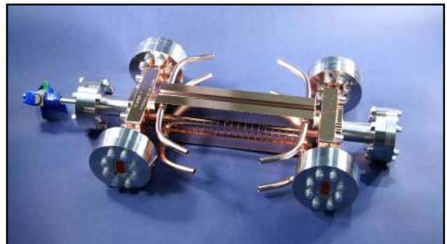
Figure 1: Photo of a KEK/SLAC made x-band accelerating structure called T18_vg2.6_disk (1).
