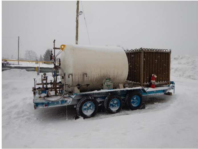
Bulk LAr storage on surface
