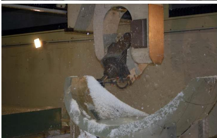
The sheets are thermoformed and machined into 'orange slices'.
