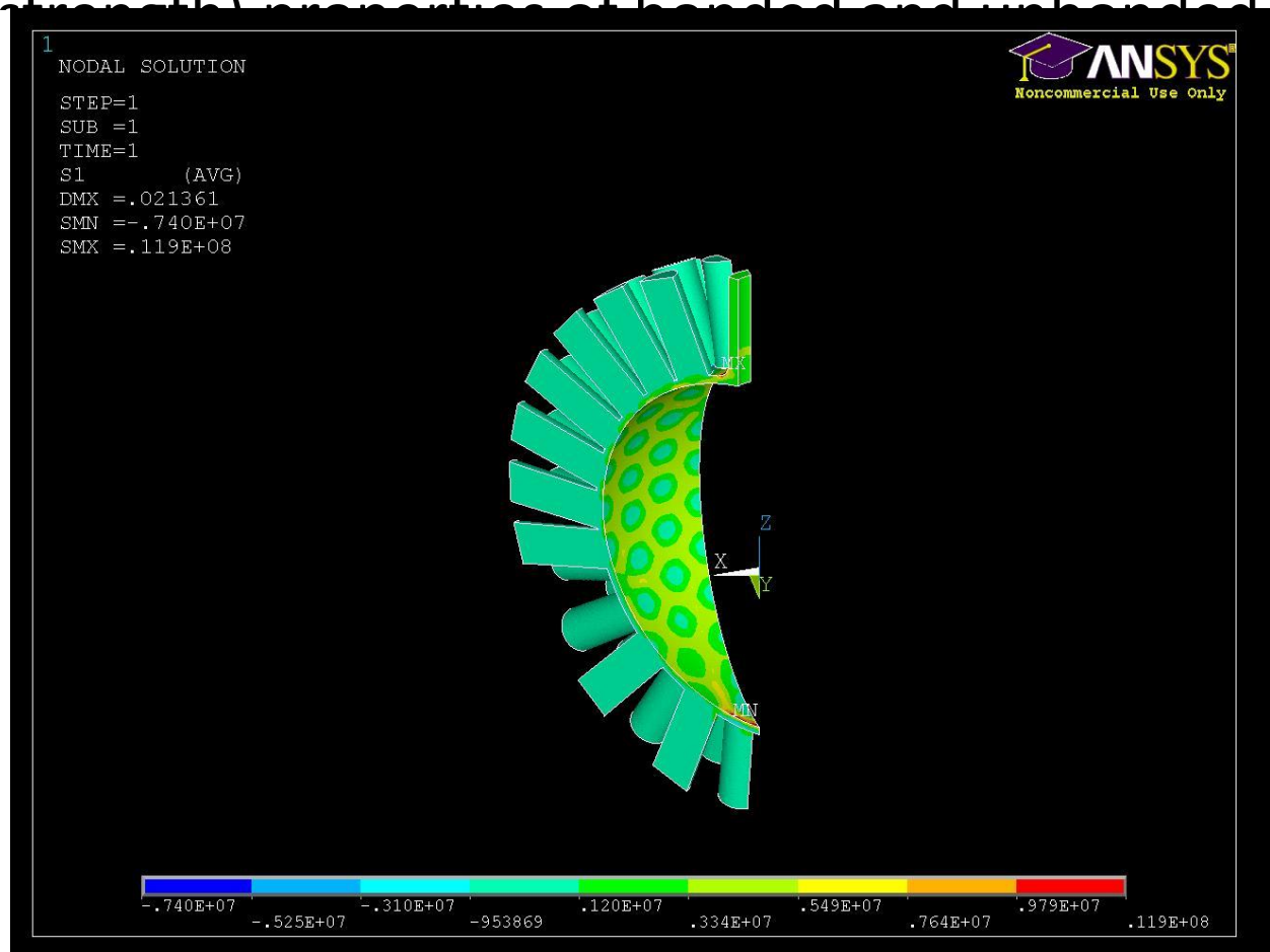
Figure 1: First principal stress for a neck and bottom supported acrylic vessel. The maximum is 11.9
