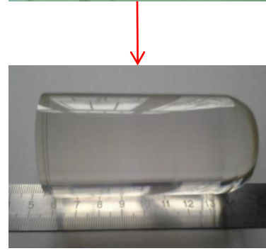
After annealing (24 h, 750° C) optical properties were restored
