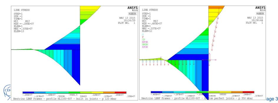
• HL1100-607 : beam – joint stiffness calculated and accounted for in FEA
