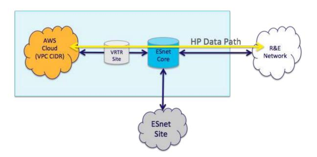
Virtual "Site Router" improves path efficiency and takes pressure off of the site local-loop.
