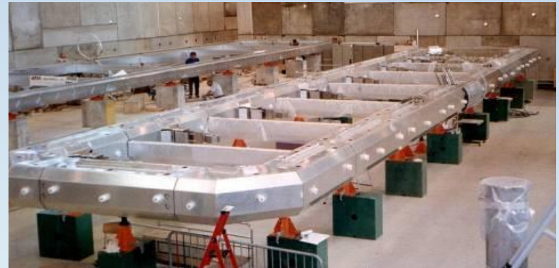
Aluminium thermal shield for the ATLAS detector at CERN
