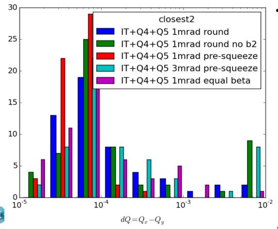
inserting the skew correctors at a location of equal beta (53.37 m from IP, IT+Q4+Q5 1mrad equal beta) helps, but still some cases with an insufficient convergence -> equal beta functions for Beam 1 and Beam 2 improves the correction, but there are still cases with an insufficient convergence
