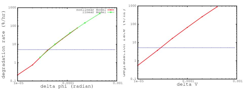
In order to have a good luminosity lifetime  $\sim 20$  hours, the noise amplitude needs to be kept below the level of a few  $10^{-5}$ .
