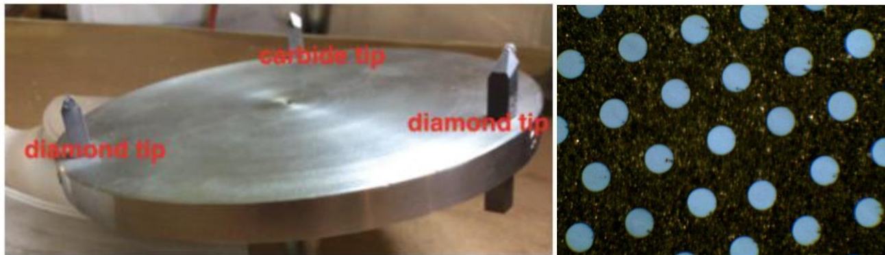
Figure 2.5. Left: Fly cutting tool used at UIUC to finish the ends of the fibers. Right: Fibers ends after fly cutting step.
