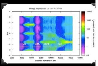
May be able to find a configuration of inner triplet optics and elliptical apertures that losses will have a favourable pattern, allowing us to significantly decrease  $\beta^*$
