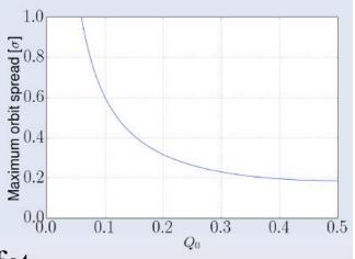
5 ns leads to several sigma effect at IP - quite severe - will need bunch by bunch orbit correction to mitigate this
