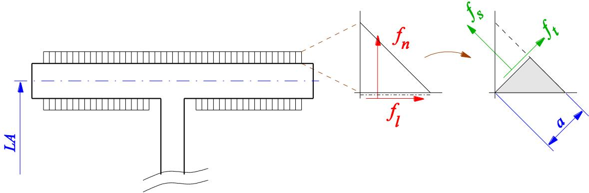
In order to simplify, we assume the moment  $M_0$  as the *only* loading, and we neglect the *web* welds. The loading to the flange welds, again somewhat simplified :
