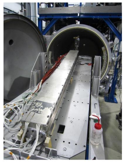
The mold is place into the tank, there are 4 couples of heating cartridges control by 4 sensor of temperature. We added a filter just before the injection point of the mold to avoid problem in case there is particle drain by the resin.
