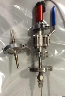
We place a Pirani sensor on the channel of injection tube to measure the vacuum level into mold before the injection of the resin. We observed a difference of factor 10 or 100 on the vacuum level of the mold and the chamber. (chamber 1\*10-3mbar mold 1\*10-1mbar).
