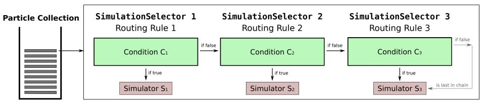
One routing chain per sub-detector volume
