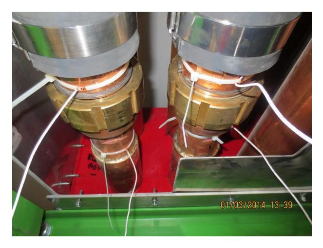
Preparation for the voltage taps test
