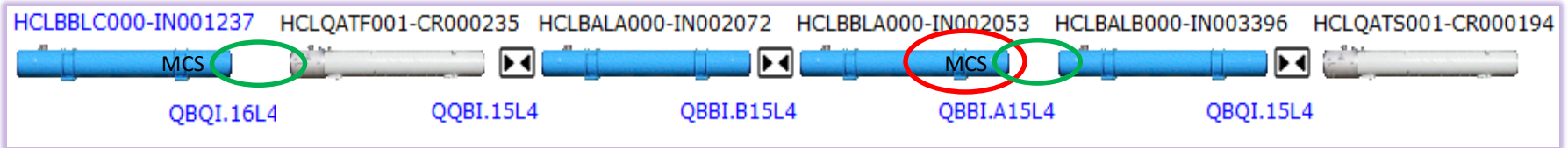
Fault located in one of this MCS leads
