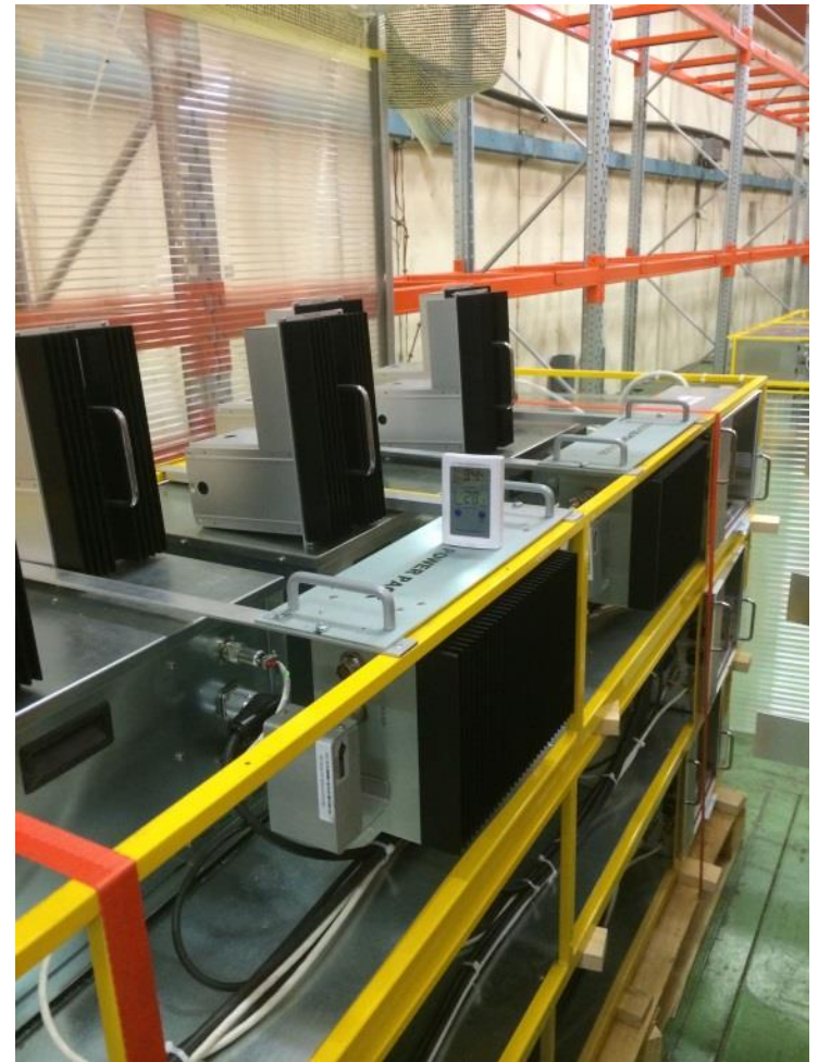
Crates have been opened up for better exchange with the blown air.
