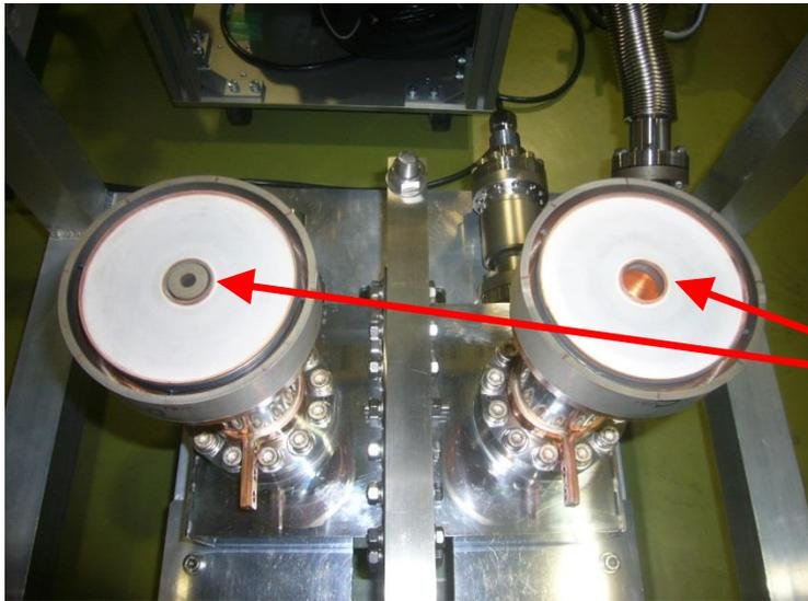
Leak at brazing of inner conductor
