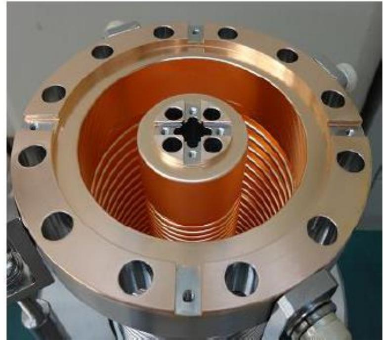
Large size of swellings ( $\phi$  5-10 mm) were formed after brazing at 800°C. The cause was inadequate plating parameters on plating area (S) and volume of solution (V) in case of Au-strike: Large bath (V) for acid solution is important, because of constant current density.
