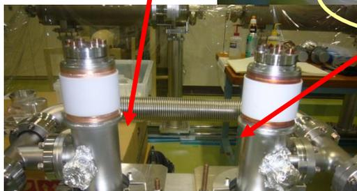
After disassembly, traces due to RF discharge were found.
