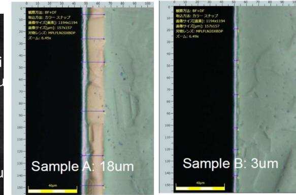
Cross-section of Cu plating
