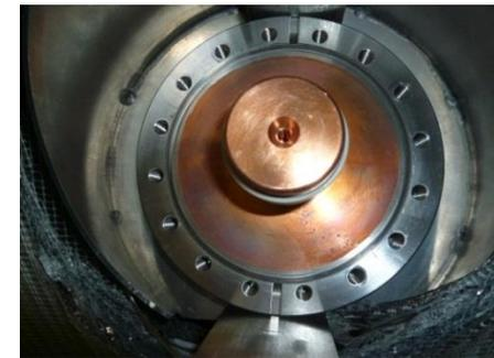
Discoloration of Cu plating in TTF-3 input couplers from DESY and FNAL
