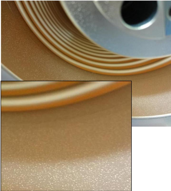
**Micro-projection ( $\phi 100\mu\text{m}$ )** were formed after brazing at  $800^\circ\text{C}$ . The cause was organic carbon contamination in an old solution.
