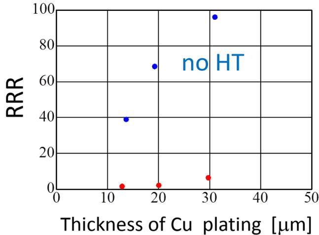
After 800°C HT in Hydrogen Furnace
