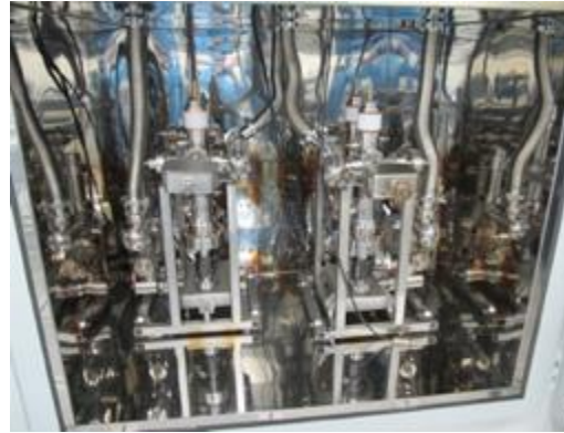
75h baking cycle at 150° C
