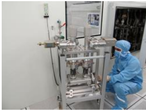
Leak test after reception
