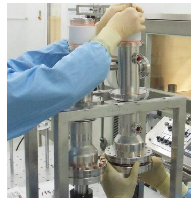
coupler pair clean room assembly, leak and actuator displacement test
