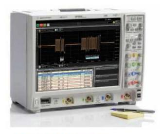
Agilent DSO 9254A 2.5 GHz bandwidth 10 Gs/s 8 bit > 1000 samples 4 channels Maximum rate ~100 Hz
