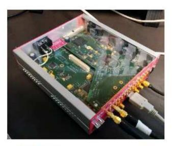
SAMPIC 2.5 GHz bandwidth 10 Gs/s (used at 6.4 Gs/s) 11 bit 64 samples 16 channels Maximum rate ~500 kHz
