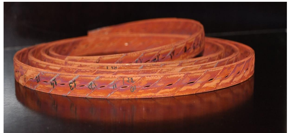
15 BHTS tapes (0.14 mm), 2 m Expected I_C (4.2 K, 20 T) \approx 5.1 kA
