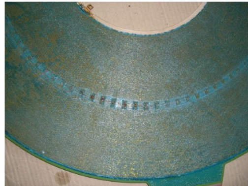
BSCO impregnated pancake, by courtesy of P. Tixador and A. Badel
