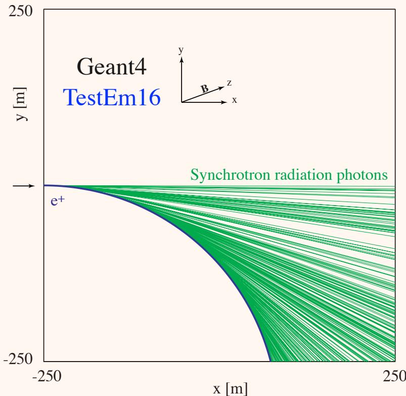
10 GeV e+ moving initially in x-direction, bend downwards on a circular path by a 0.1 T magnetic field in z-direction. [Geant4](#) TestEm16
