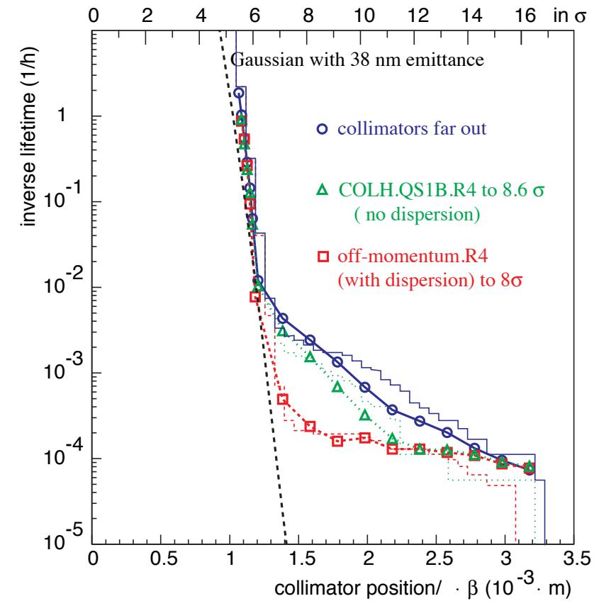
Tails from : beam-beam, high chromaticity, particle scattering
