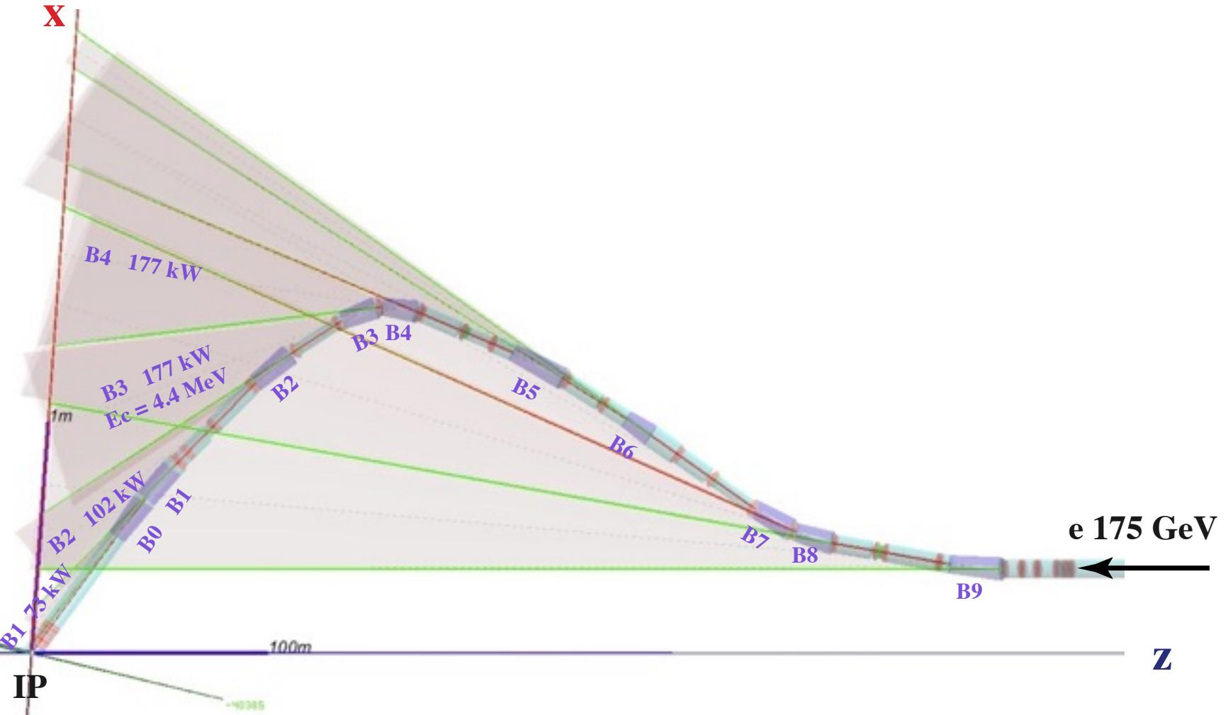
**Synchrotron radiation into IR major challenge : 0.6 MW / beam of MeV  $\gamma$ 's into detector region**
