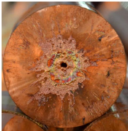
Effect of the SPS beam exiting a 60 cm copper cylinder [1]
