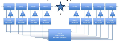
Proposed CC LLRF architecture for one ring and IP [3]
