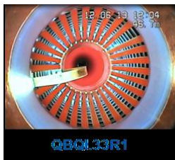
A non-conforming RF insert [6]
