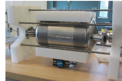
499 MHz Set Up for Trimming
