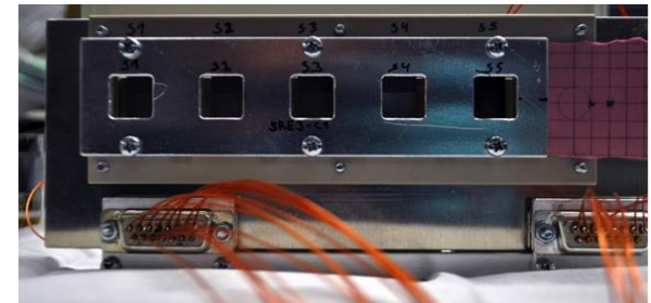
Sample holder for R measurements
