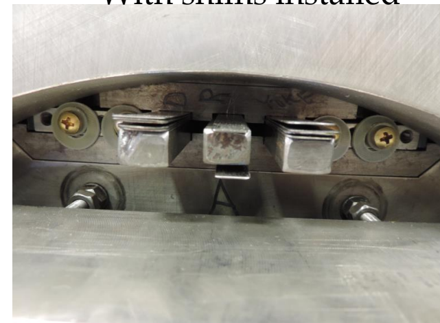
With shims installed
