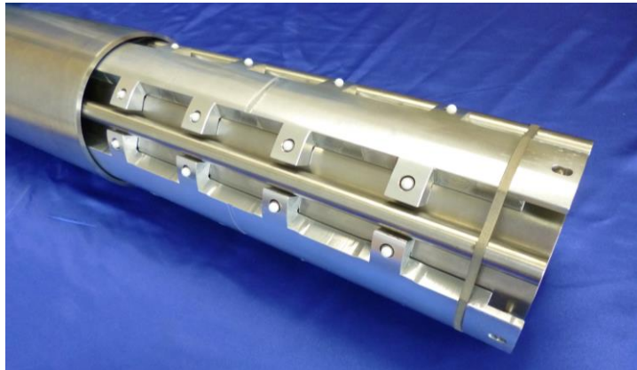
Beam screen assembly
