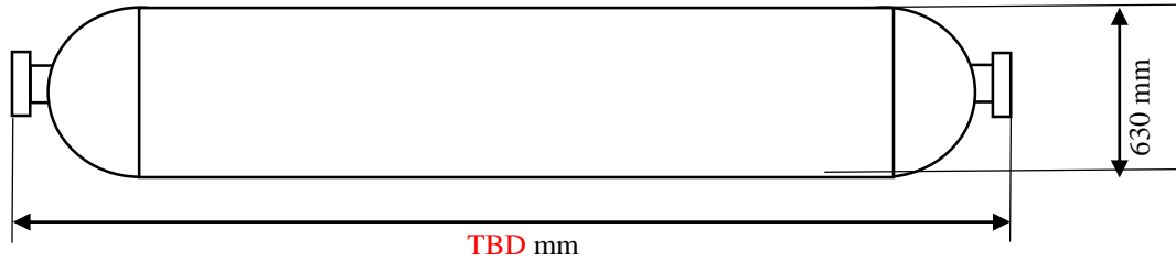
Figure 4: LMQXFA/B Physical Envelope Dimensions
