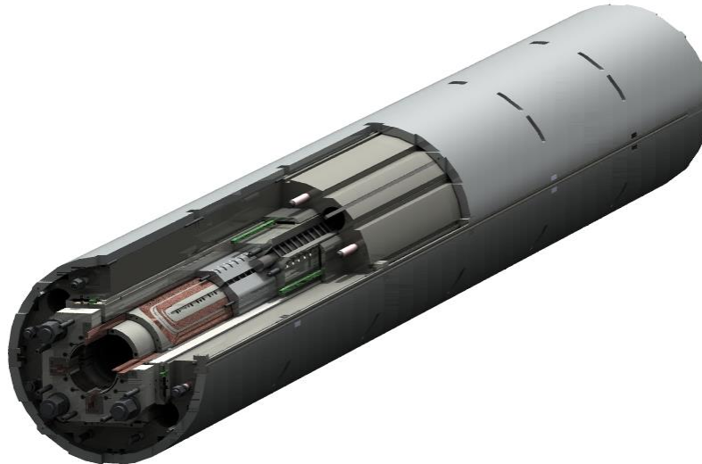
Figure 4: MQXFA 3-D conceptual cutaway view
