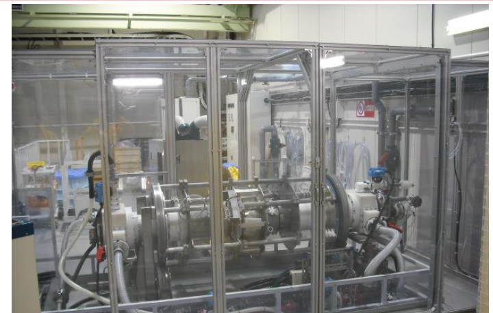
Our EP apparatus for 500 MHz cavity 46
