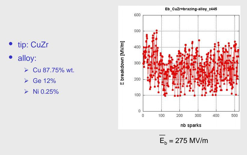
no degradation due to alloy (even better than pure CuZr, ~ 130MV/m)
