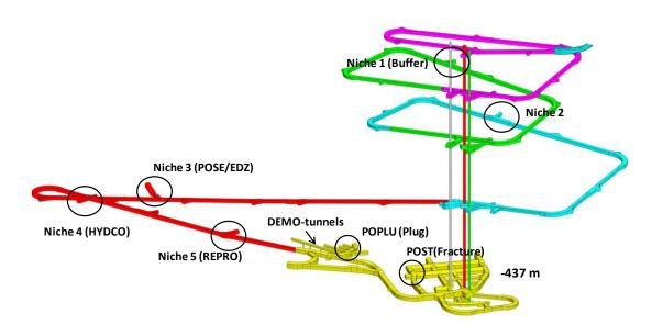
Figure 1 – Layout of the ONKALO facility and locations for different *in-situ* test sites.
