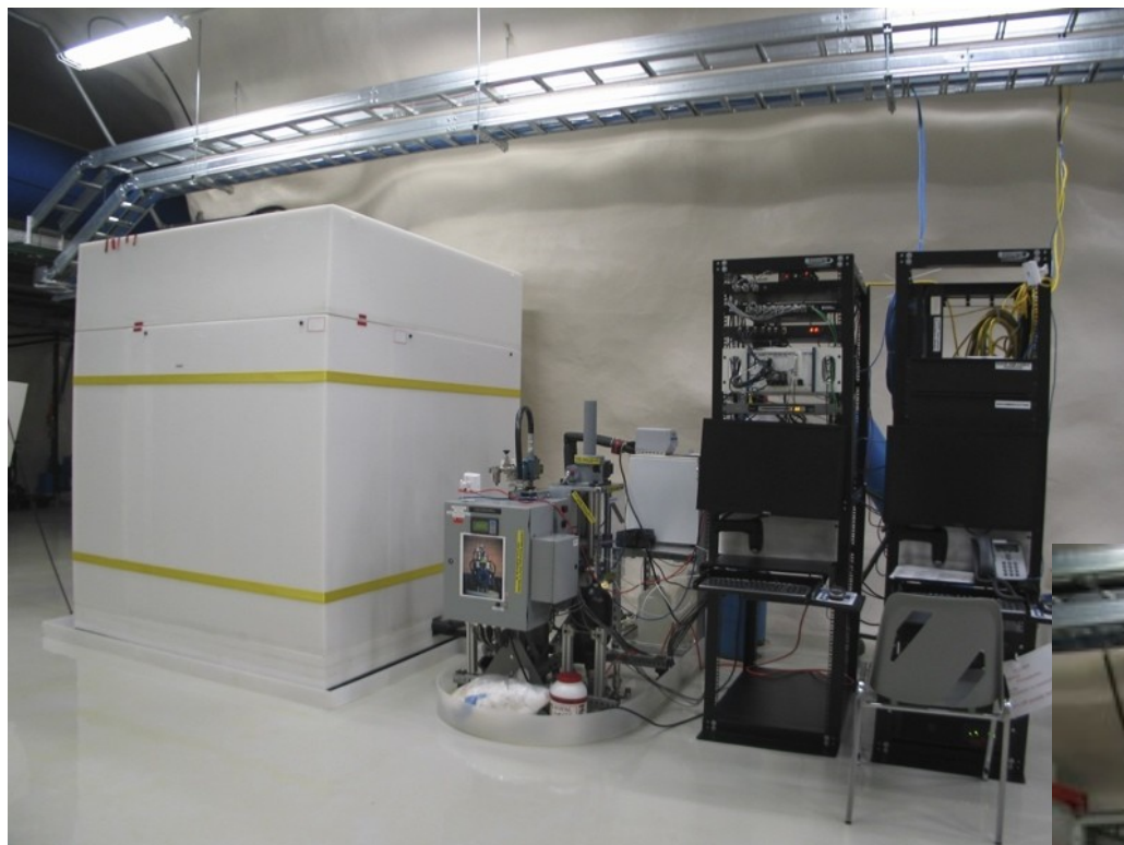
PICO-2 bubble chamber, showing water tank shielding stack, pressure carts, DAQ racks
