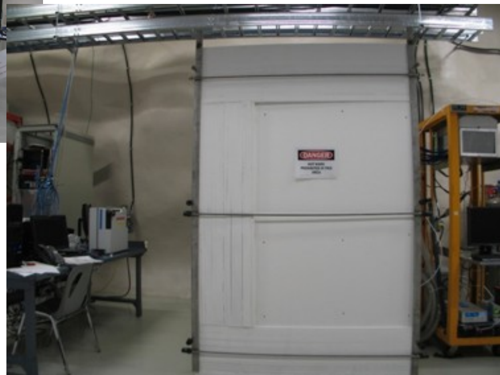
DAMIC CCD-based dark matter detector, focus on low mass WIMPS. (Currently 10g target, increase to 100g expected)
