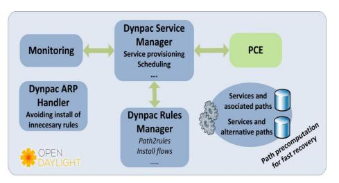
DynPaC Service Manager asks the PCE for a path between the source and destination nodes, accordingly with the available bandwidth and topology.
