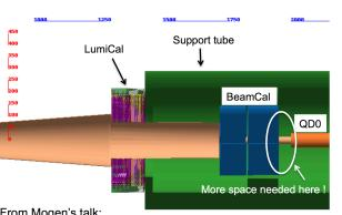
Removed LHcal. For Lumical and Beamcal: kept dimensions of the ILD design.
