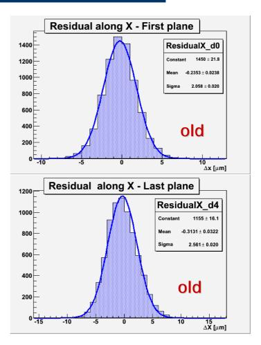
Precision of alignment better than 0.05 μm!
