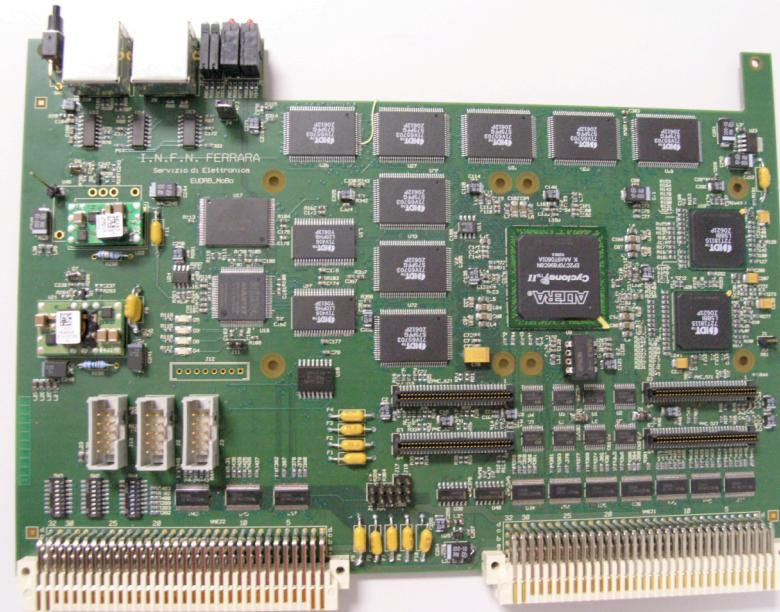
mother board built around an ALTERA CycloneII FPGA (clock rate: 80MHz) and hosting the core resources and Interfaces ([VME64X slave](#), [USB2.0](#), [EUDET trigger bus](#))
