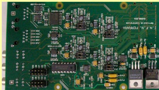
digital daughter card drives/receives control signals for the detectors and features a USB 2.0 link
