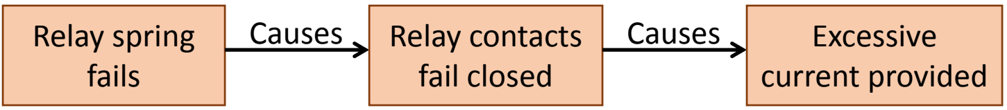
Accident model: Chain-of-failure-events
