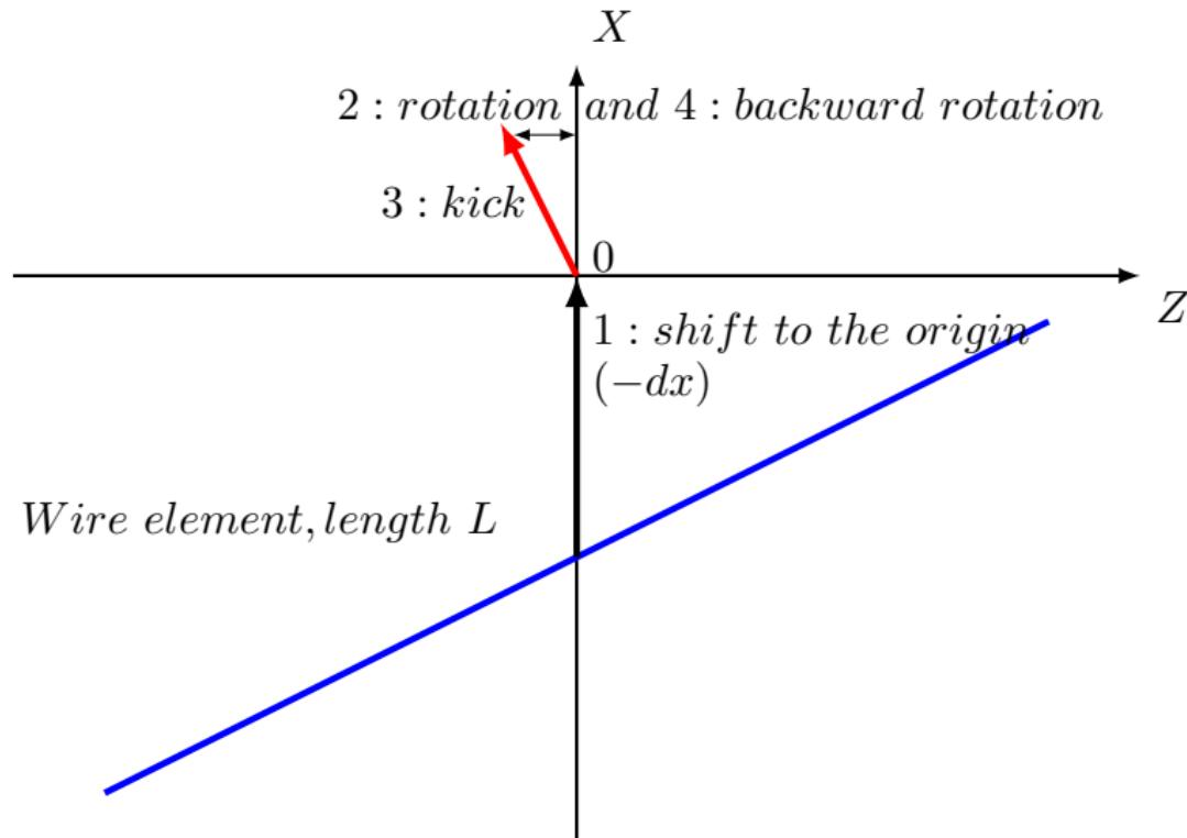
NOTE:  $L$  - emb. drift; kick is a function of  $L$  and wire length  $l$
