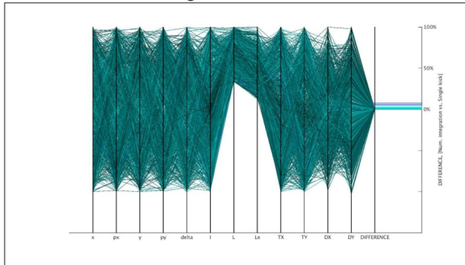
The axis on the right shows the difference between models (in %) for arbitrary combinations of the variables:  $x, px, y, py, \delta$ , tilts:  $tx, ty$ ; and displacements:  $dx, dy$ . The limitations were:  $x \ll L, px \ll 1, dx < L$ . 20000 of combinations are shown; 99.8 % of cases provides the difference  $< 0.1\%$ ; in a few cases the difference is about 1-5 % and can be explained by numerical rounding, when the angles is close to 90 degrees.
