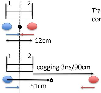
Traces from Port 1 and Port 2 overlaps in time. Strong correlation between Beam 1 and Beam 2 positions.
