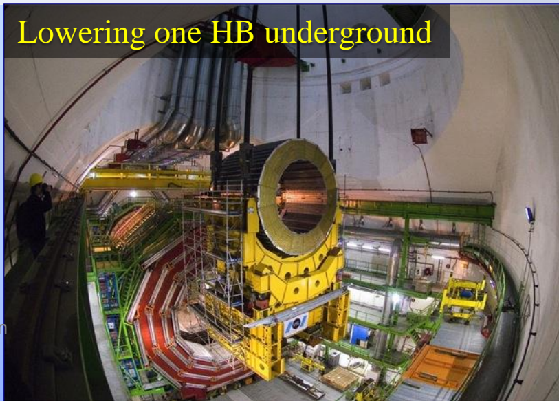
HB+ about to be inserted into YB0
