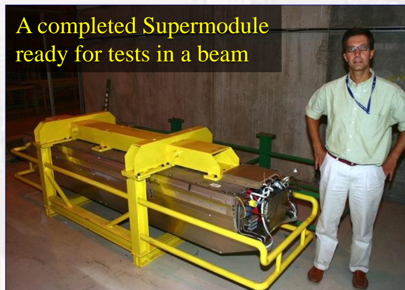
An ECAL Module of 400 crystals
